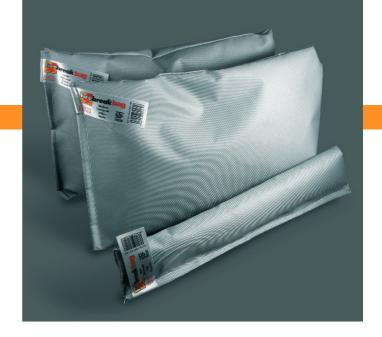
Firebreak Bags comprise a range of different sized coated glass cloth bags filled with a blend of durable intumescent and inert fillers. They are designed to be installed around services in penetrating fire resistant walls to provide either a temporary or permanent fire seal of up to 120 minutes.
